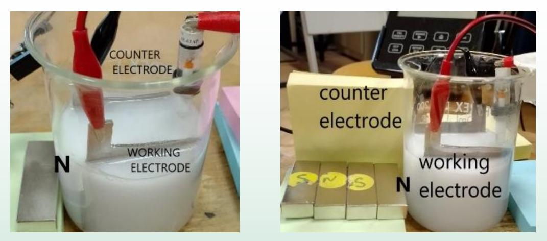
Experiments were conducted in beaker. Cyclic voltammetry scans measured for all the solutions in the absence and presence of magnetic field (MF).
