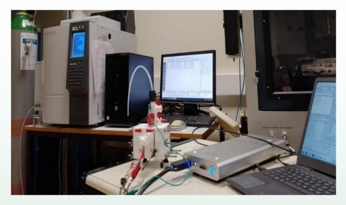
Experiments were conducted in the above custom-made seawater electrolysis cell. Hydrogen production was monitored by GC, under the same potential values (-1.95V, -2.1V) for all seawater solutions. NaOH enhancement was tested for 4%, 10%, 20%, 30% & 40% wt. The effect of magnetic field was also examined and evaluated.
